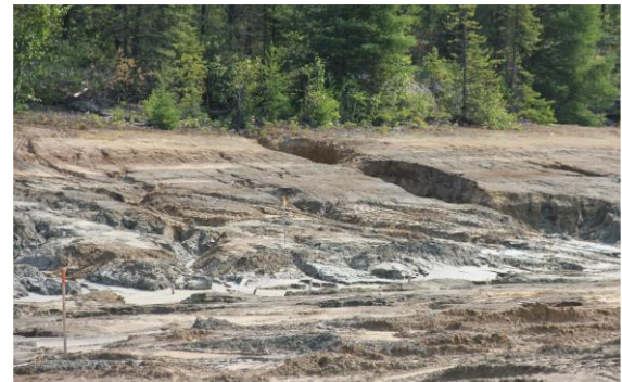
Mine tailings in contact with air subject to strong erosion and generation of leachates that are toxic to the population.
