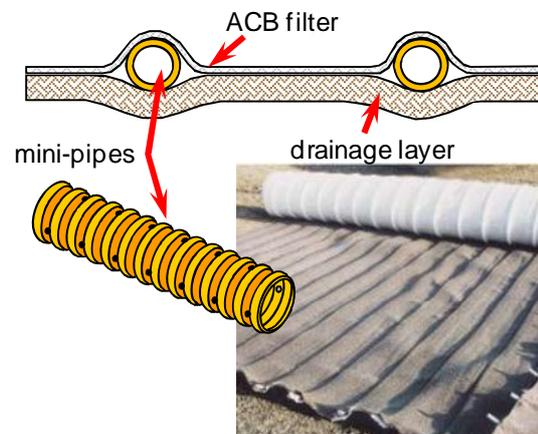
Figure 2. Tested drainage geocomposite
