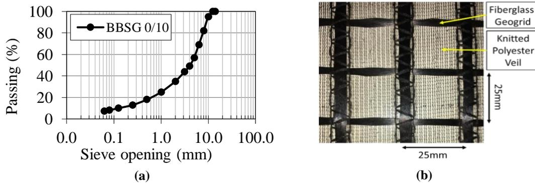
**Figure 1. Components of tested specimen: a) Bituminous mixture gradation curve and b) fiberglass geogrid Notex Glass® C 50/50**
