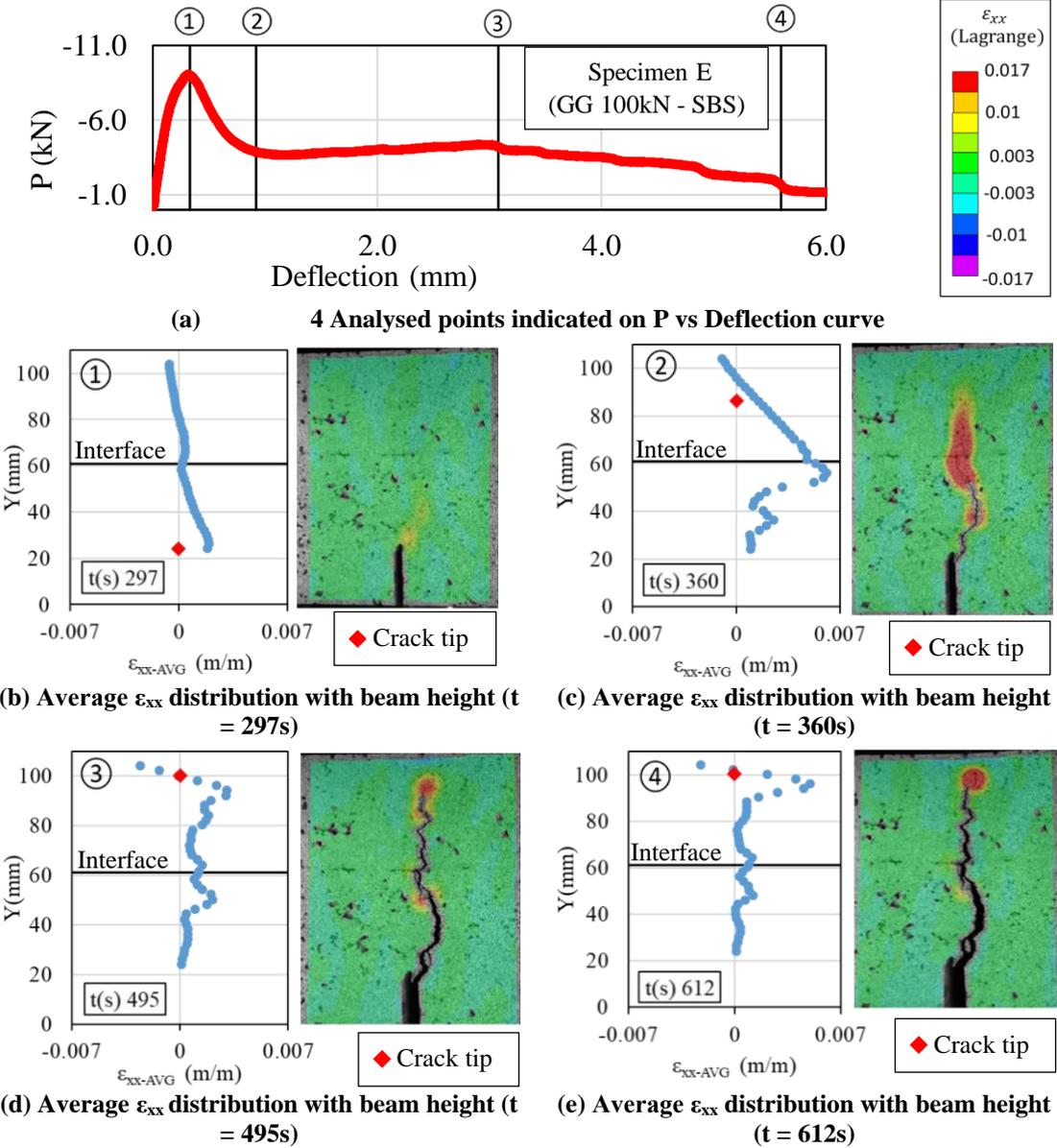
**Figure 6. DIC analysis for specimen E (Notex Glass® C 100/100-25, emulsion SBS) at points 1, 2, 3 and 4**
