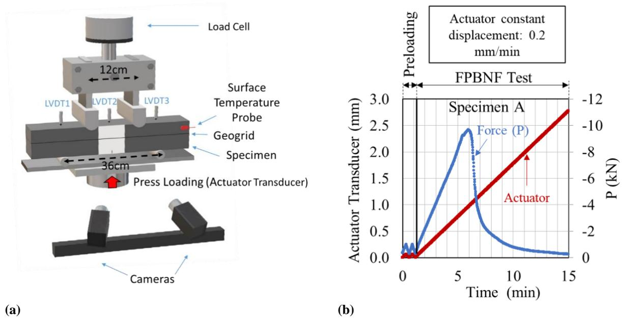
**Figure 3. Experimental test device and procedure for FPBNF: a) scheme and measurement device location, b) Actuator displacement and force versus time during the test on specimen A**
