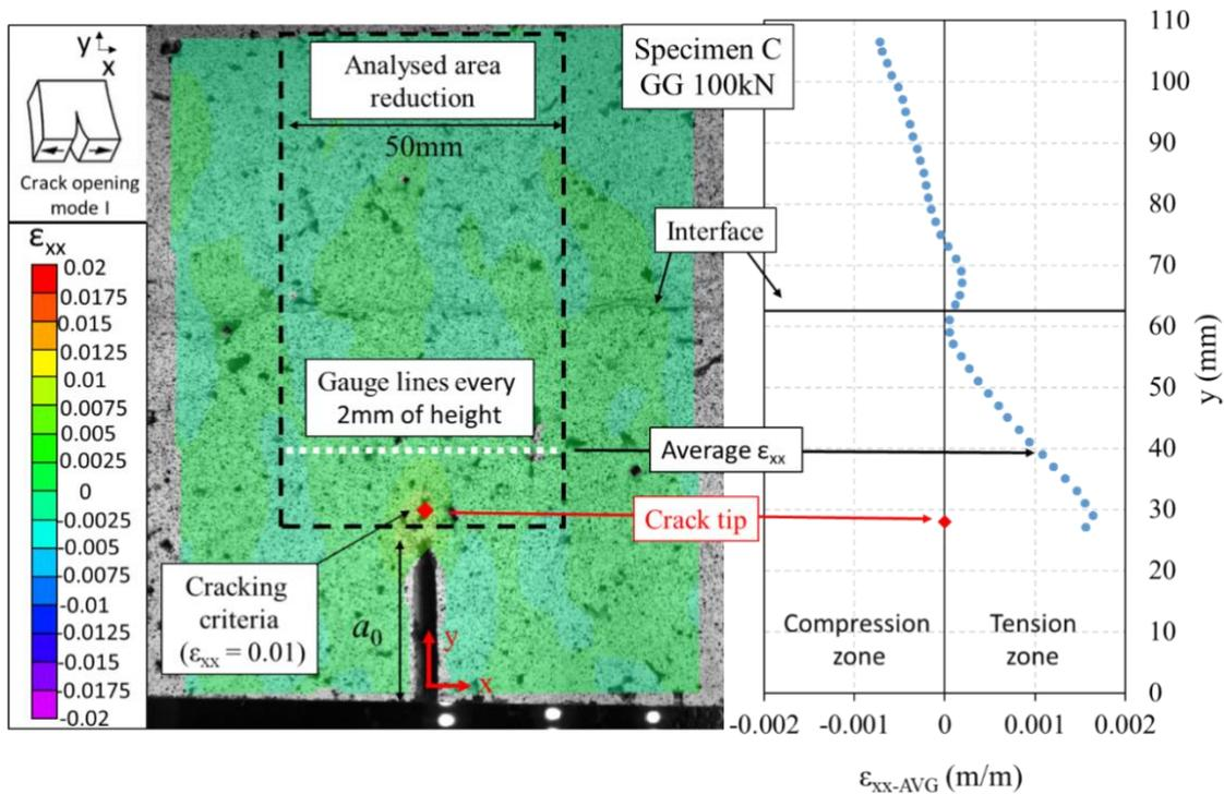
Figure 4. Explanation of analysis performed from data obtained with Digital Image Correlation (DIC) using Vic-3D 7 software
