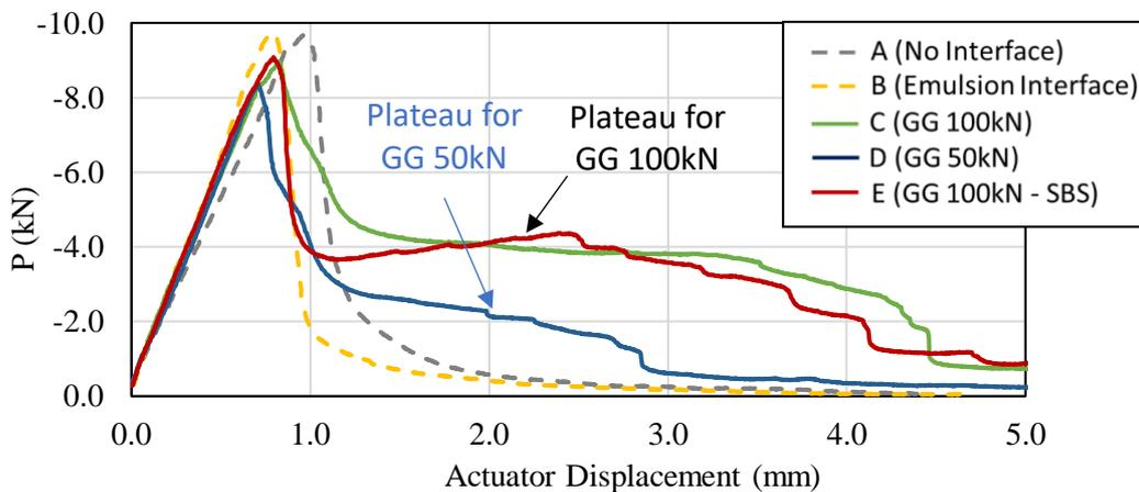
Figure 5. Force vs Actuator Displacement for all tested specimens
