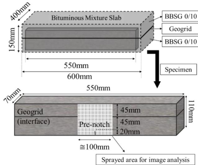
**Figure 2. Bituminous mixture slabs obtain with French wheel compactor and beam specimen obtained from sawing**
