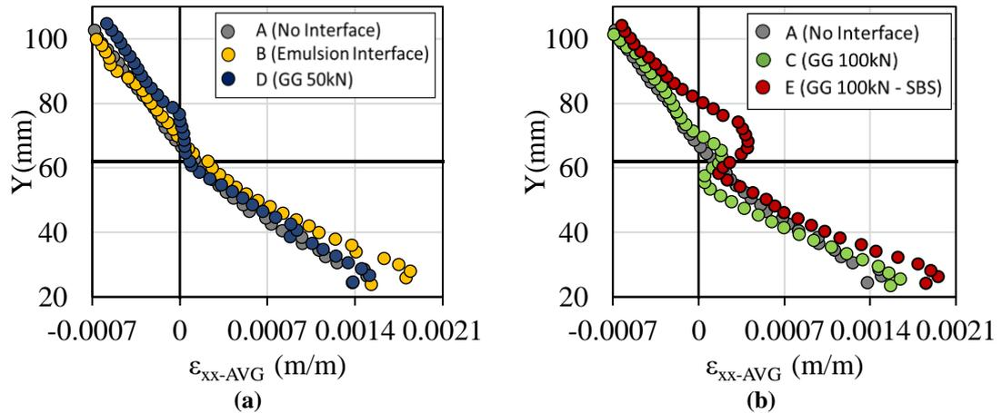
**Figure 7.**  $\epsilon_{xx-AVG}$  at different heights for the five tested specimens at peak load point (point 1 in figure 6)
