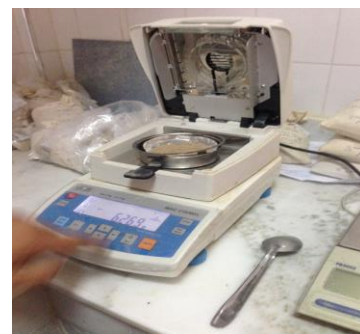
Figure 10: Measurements using the desiccant scale
