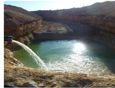
Figure 19: Opening of the collector of the bottom of the test basin.
