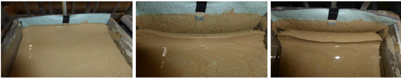
Figure 11: Surface condition after filling, after 8 h and after 22 h
