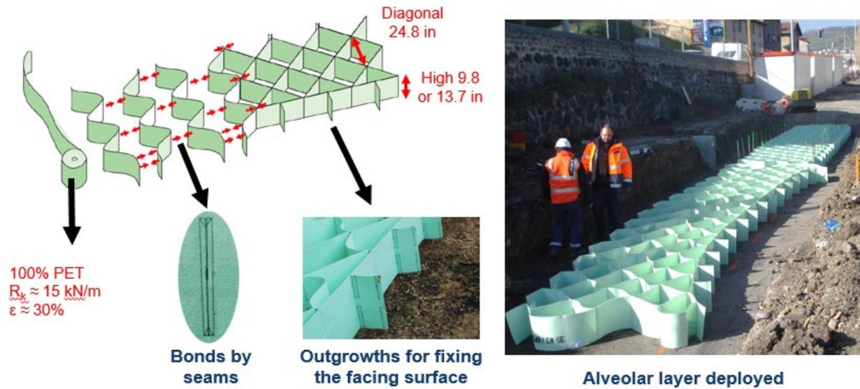
Figure 3. Details of the Geosynthetic geocells M3S.
