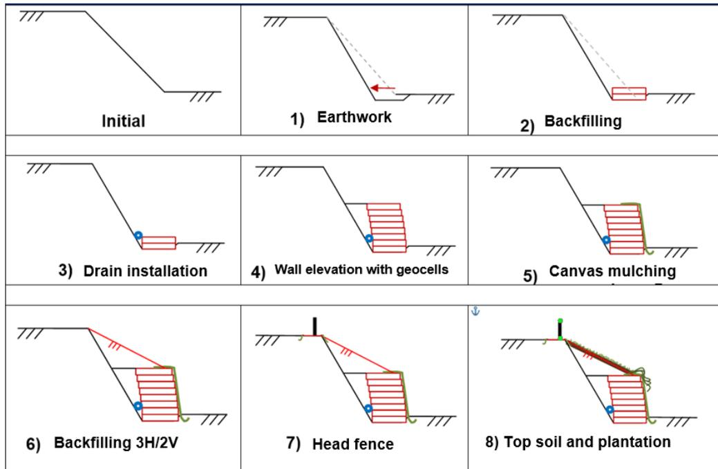
**Figure 5. General phasing of reinforcement work.**
