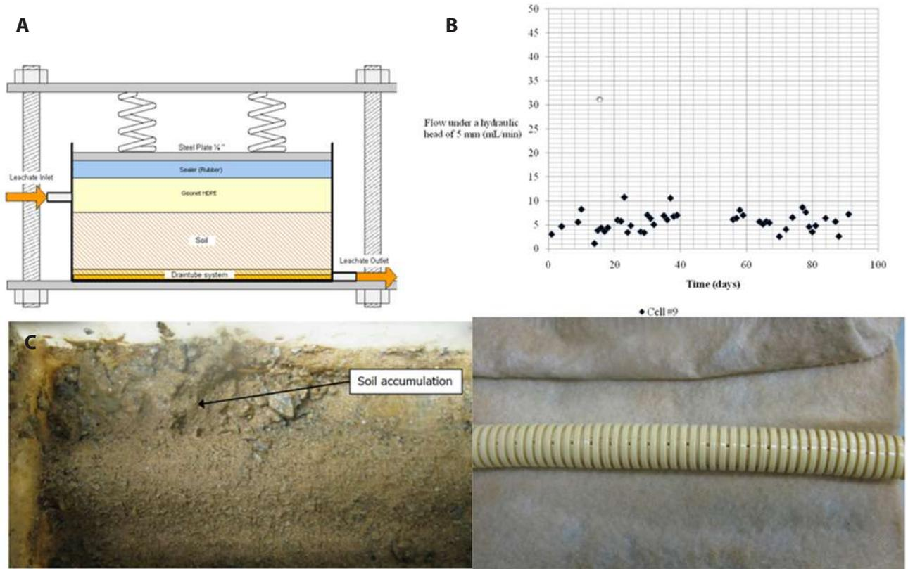
**FIG 10** – Draintube™ geocomposite behaviour during long-term flow test with copper ore (after Blond and Saunier, 2014): (A) schematic cross-section of the experimental leaching cell design; (B) flow rates evolution over time under a hydraulic head of 5 mm (see Blond and Saunier, 2014); (C) external (left) and internal (right) view of the geocomposite after three months of sulfuric acid percolation.
