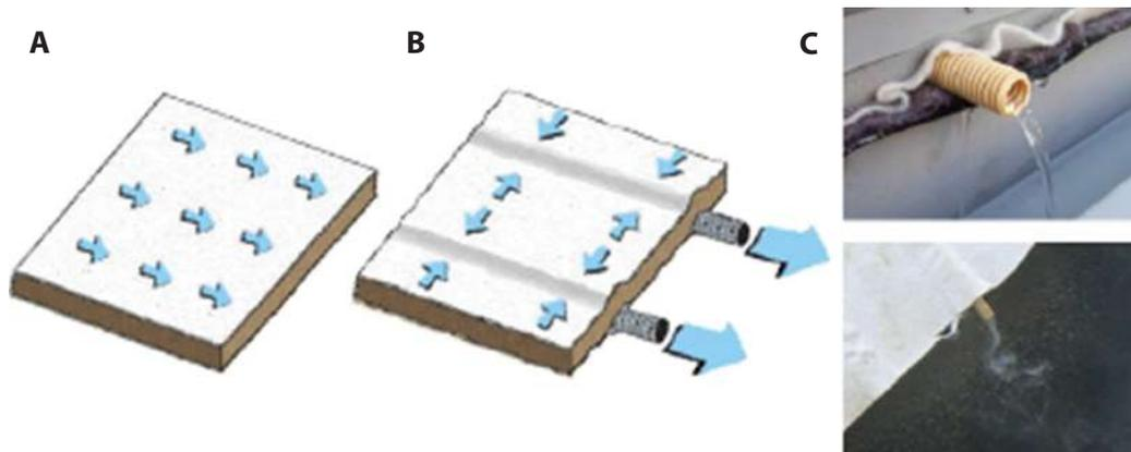
FIG 2 – Hydraulic functioning of the DRAINTUBE™: (A) flow in a homogeneous layer (direction of the slope); (B) flows in the DRAINTUBE™ geocomposite (mini drains direction); (C) photos of field installation of DRAINTUBE™ geocomposite with fluids discharge.
