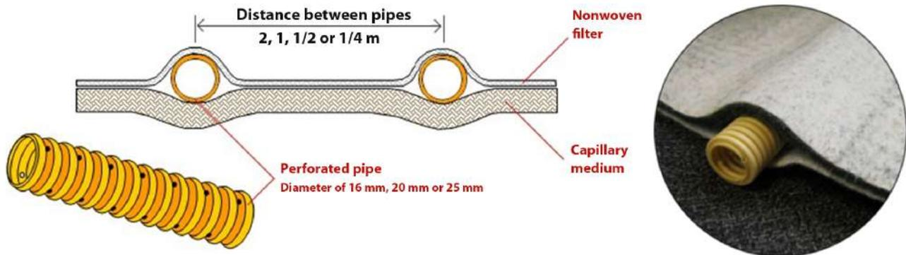
FIG 1 – Afitec DRAINTUBE™ geocomposite: a schematic of the structure (left) and photo of the DRAINTUBE™ (right).
