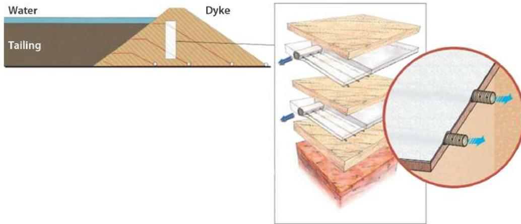
FIG 7 – Design schematic of the DRAINTUBE™ as a barrier for dry tailing of mining waste materials.
