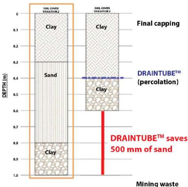
FIG 8 – Profiles of soil cover geometries (AMEC, 2011) over the Central Manitoba Mine, Canada, abandoned tailing. Left profile: traditional approach with sand used as drainage material. Right column: DRAINTUBE™ replacing the sand material.
