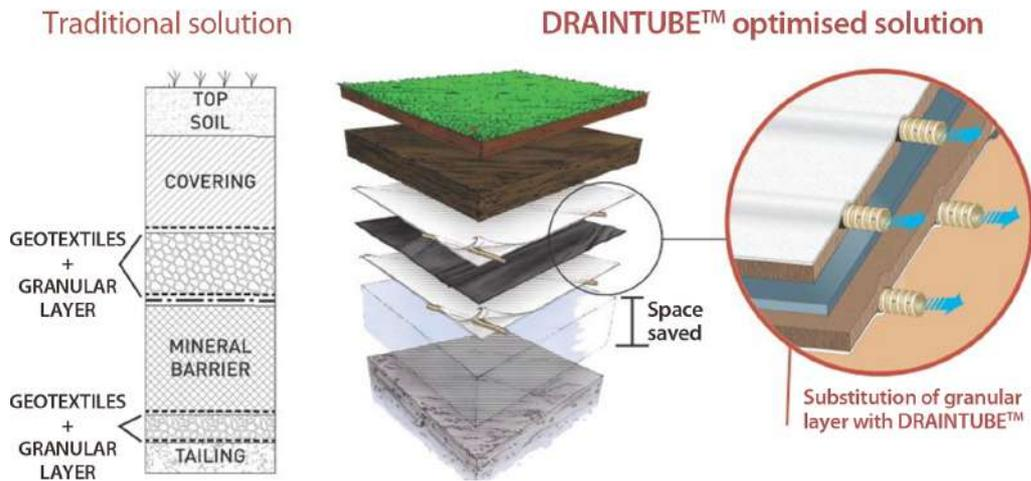
**FIG 5** – Design schematic of the DRAINTUBE™ for covering of tailings.
