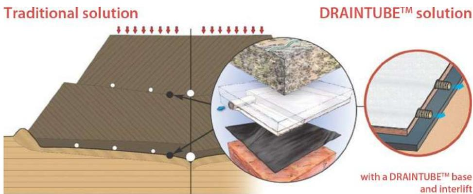
**FIG 6** – Design schematic of the DRAINTUBE™ for heap leach pads.
