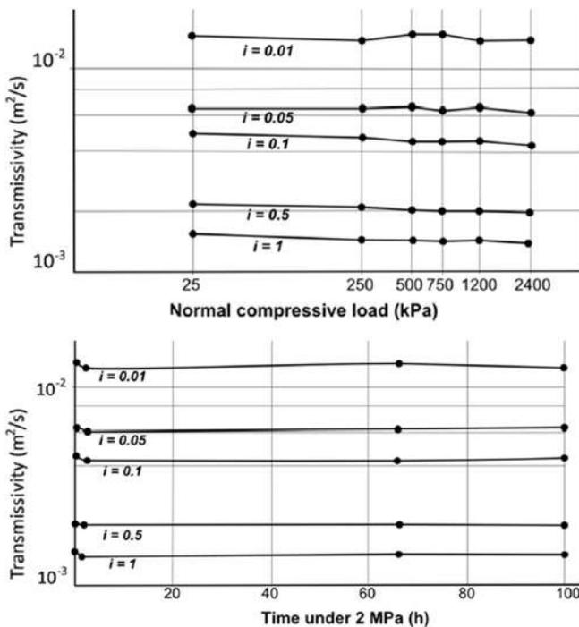
**FIG 11** – Draintube™ geocomposite behaviour under high compressive load (after Saunier and Blond, 2010).
