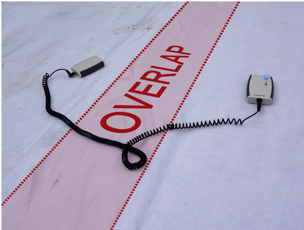
Figure 5: Continuity tester for quality control
